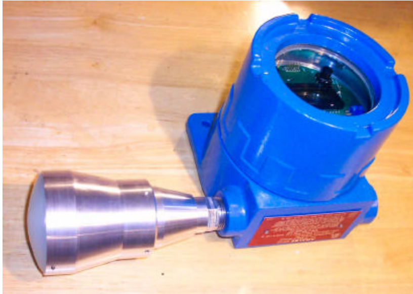
Fig. 1. Velocimeter with 3 inch lens-horn, 4.5" cylindrical housing.
